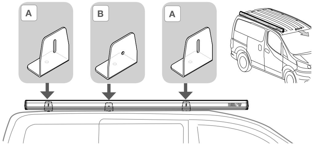
**EN** Before tightening the screws, make sure that the awning position doesn't prevent the opening of the rear door.
